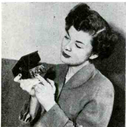
The Olson speaker on an RCA portable. V-shaped cutouts act as reflex ports.
