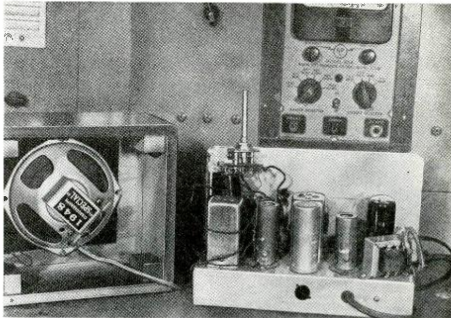
This 4-tube receiver has high performance. Note feedback loop around i.f. can.
